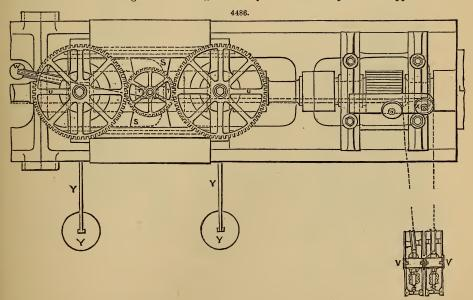
upper end by the wrought-iron standard S, between the housings, and in the centre of the length of the rolls. On the top of the shaft is keyed a spur-wheel T, which drives the two spur-wheels U U on the vertical holding-down screws of the top roll R. These screws work in steel
